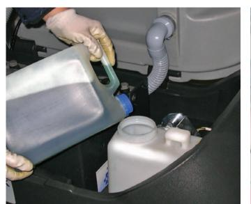
3. Fill the EcoFlex<sup>™</sup> tank with a detergent suitable for the work to be performed (highly concentrated detergent).
