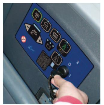
**3** Turn the ignition key to "0", then try to start the machine without pressing the paddle.
