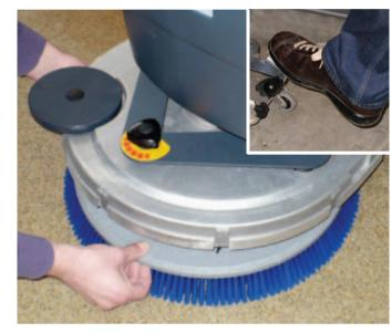
5. Place the brush or the pad-holder under the deck. Use the appropriate brush to clean the floor. Lower the deck by pressing the pedal deck.
