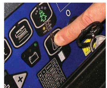
8. Press the detergent flow control switch. The number of display shows the detergent concentration level in the solution (see the table on the label).
