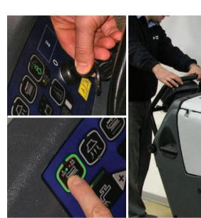
6. Turn the ignition key to "I", then start the machine by pressing the Green switch. To engage the brush, slightly press the drive paddle and then release it.
